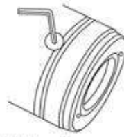
Tighten the cover anti rotation screws
