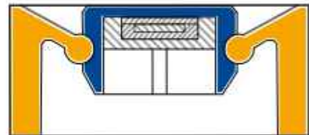
Chip in assembled state with fixing ring
